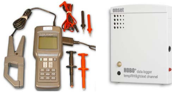
Figure 3.4: Images of the Fluke 41B and HOBOWare Data Logger used for Independent Measurements
